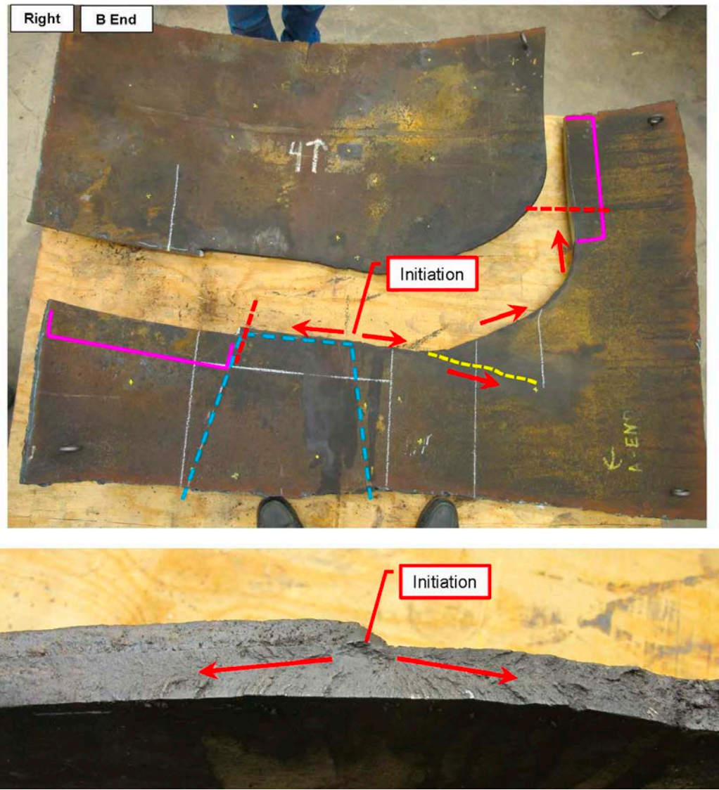
Figure 10. Interior view of the tank shell coupon.
