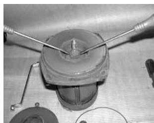
1) Detach the shaft seal using two screwdrivers. Do not damage the sealing surface of the shaft.
