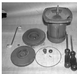
3) The motor unit disassembled, with installation tools.
