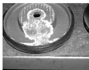
2) Also detach the sealing flange from the motor front plate using two screwdrivers. If needed, replace the sealing flange with a new one.
