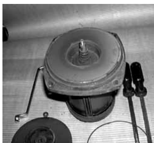
Starting situation. The motor unit with the impeller detached.
