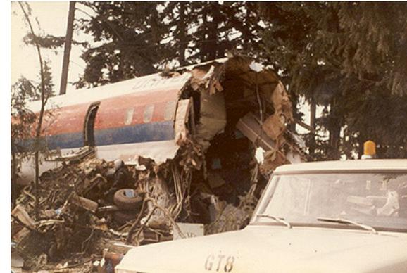
The NTSB investigation revealed that when the landing gear was lowered, a loud thump was heard. That unusual sound was accompanied by abnormal vibration and an abnormal yaw of the aircraft. The right main landing gear retract cylinder assembly had failed due to corrosion, and that allowed the right gear to free fall.
