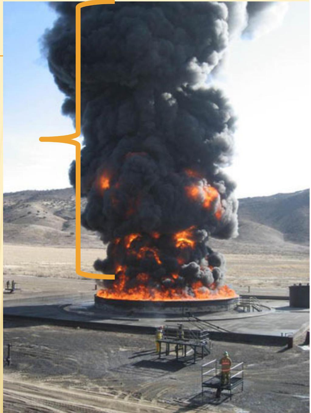
“Depending on the fuel and the size of the fire, up to 20 % of the fuel mass is converted to smoke particulate in the combustion process. This smoke shields much of the luminous flame region from the viewer, and it is this luminous flame region that is the source of most of the thermal radiation. This shielding effect is most pronounced for fires that are **tens or hundreds of meters in diameter** because of the decreased efficiency of combustion at these scales.”
