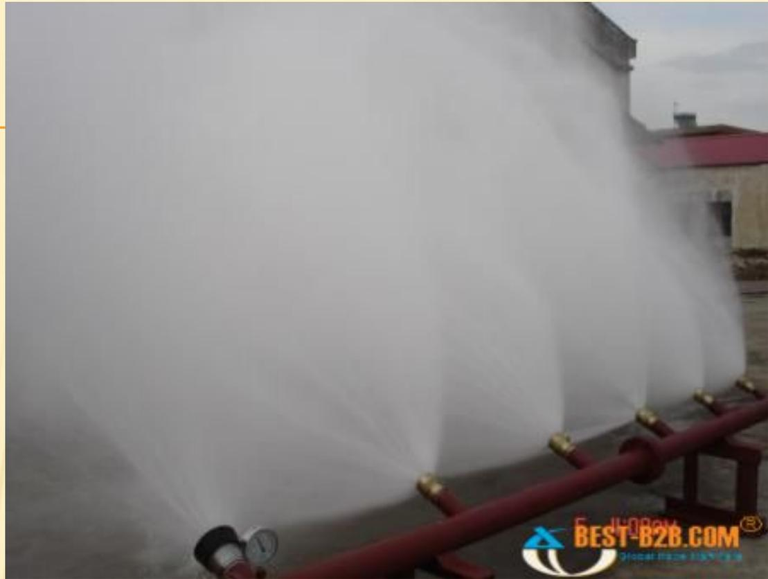
Heat transfer through a water spray curtain under the effect of a strong radiative source
